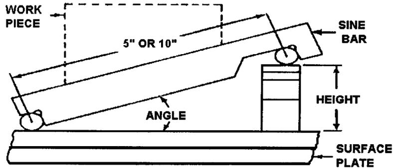
Sine bars or sine plates usually have a length of 5 inches or 10 inches. These standard lengths are commonly used by the tool maker or inspector. The sine bar or sine plate is used for accurately setting up work for machining or for inspection. Gage blocks are usually used for establishing the height.
